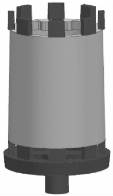
图 2 浇注系统设计 Fig.2 Design of gating system
